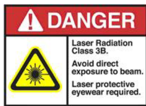
Figure 7: Laser Safety Warning Sign for Unrecommended/Non-Default Operation
